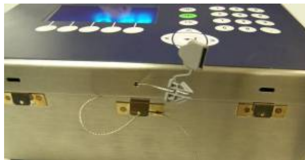
Figure 2-38: External Sealing of the Harsh Enclosure
