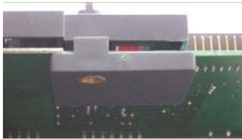
Figure 2-39: Attaching the Plastic Bottom Sealing Plate
