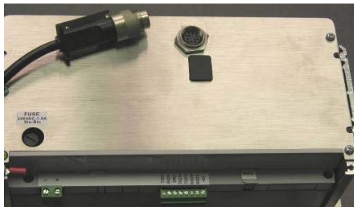
Figure 2-17: IDNet Connector Location on the Panel-Mount Enclosure
