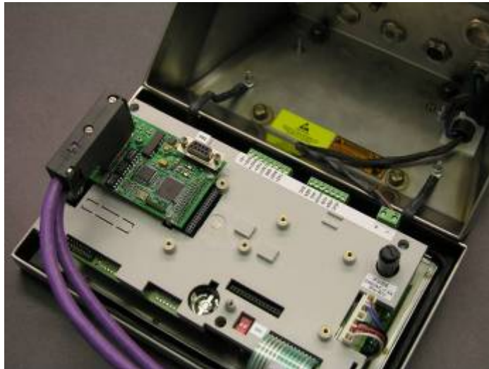
Figure 2-30: PROFIBUS Connection to Harsh Enclosure
