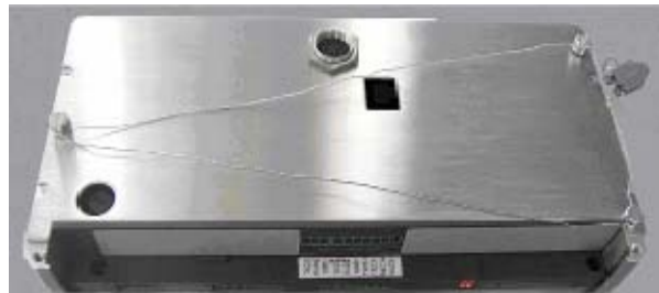
Figure 2-37: External Sealing for Canada
